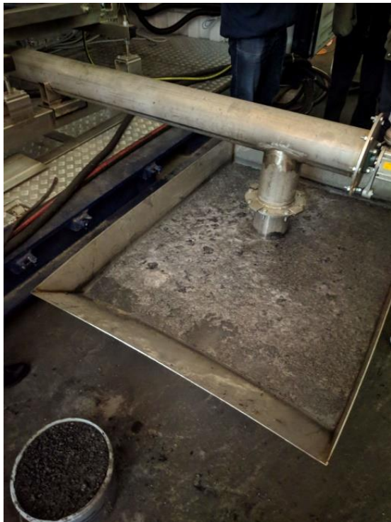
2.2 Discharge of the solid material resulting from the water bath in THE HR module
